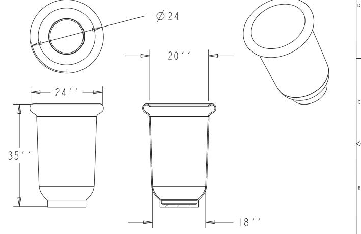
TCN-20L- Liner for trash recepticle TCN-20A- Alummum spinning for ash tray
